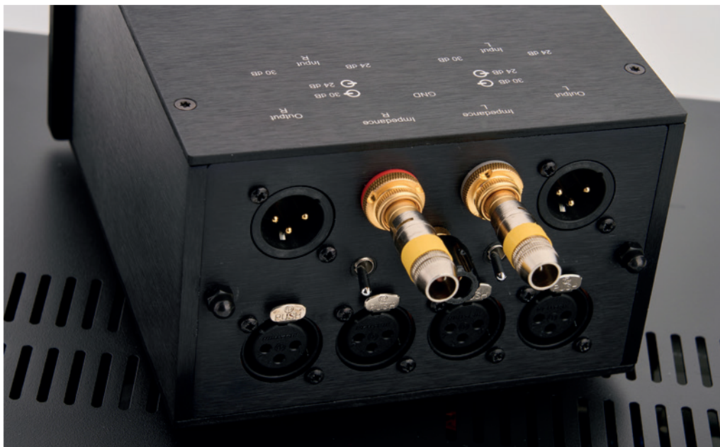
The transformer shows up with RCA plugs for impedance matching. Per channel, two inputs for signal amplification of 24 and 30 decibels respectively are designed as XLR sockets, as are the outputs
