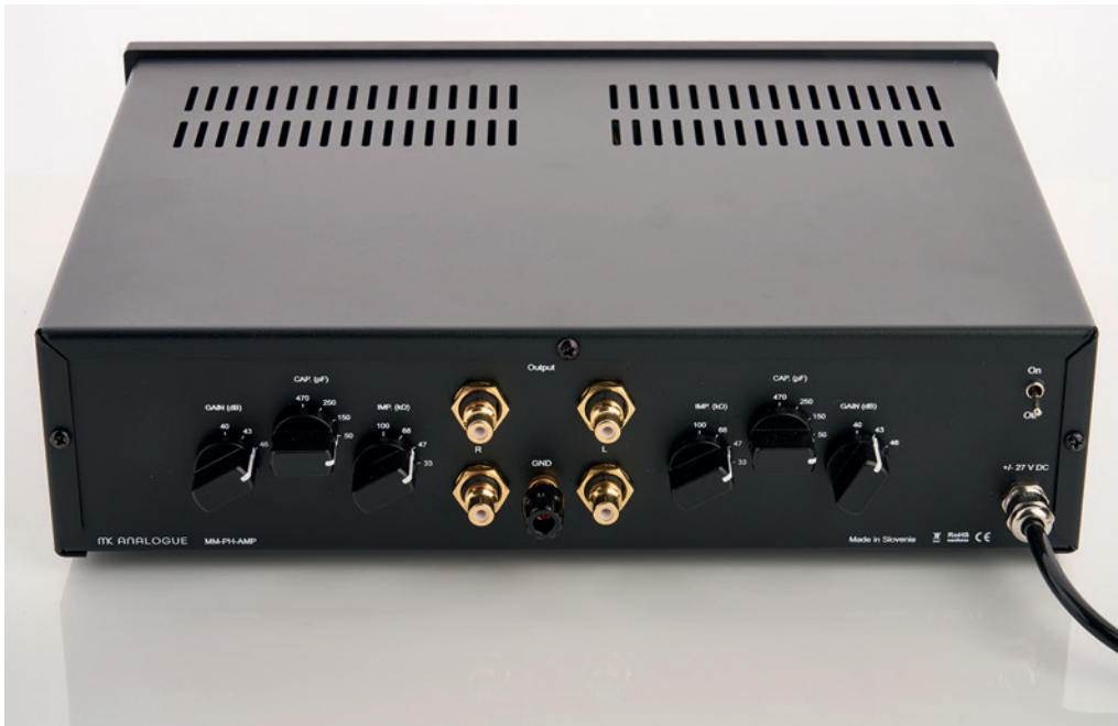
The phono stage works unbalanced and therefore only has RCA sockets
