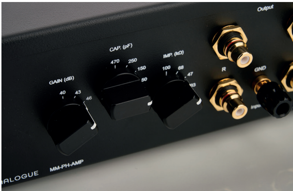
The MM phono stage not only allows to select the load capacity for the cartridge and the amplification factor, but also the input impedance
